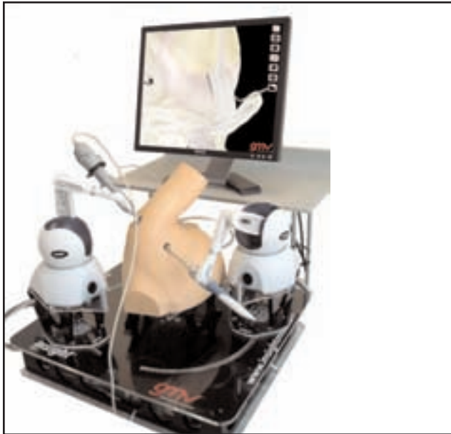
Figure 1. The insightArthroVR® trains physicians on key aspects of the arthroscopic surgery procedure.
