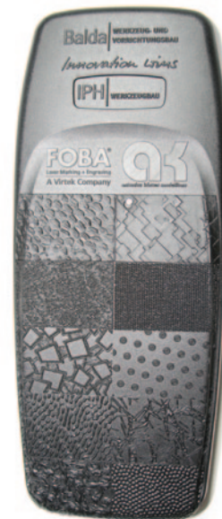
Cell phone cover with manufactured sample textures
