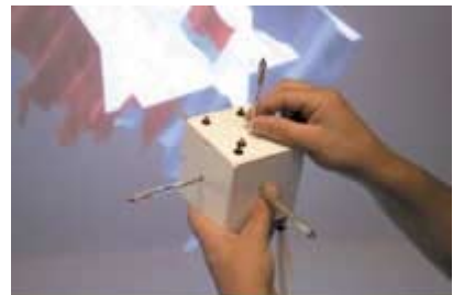
The three rods of the Fakespace/GMD Cubic Mouse set orthogonal slicing planes that can be moved through a 3D visualization to explore interior structures from various perspectives.
