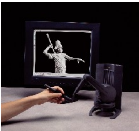
(Left) The FreeForm Modeling system enables Zack to create highly detailed, free-form shapes using the sense of touch.
